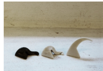
Orton-cones no. 3, 4 and 5. The kiln cooled down by 40 ° C. per hour.
