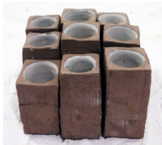
Wheeled and facet cut earthenware. Ball clay slip at the inside. Unfired
