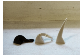
Orton-cones no. 3, 4 and 5 The kiln cooled down automatically.
